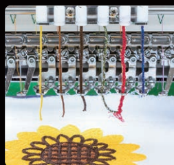
Multi cording Device 2 Embroidering 6 various types/colors of cords
